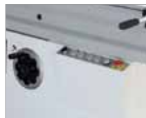
Electric saw blade height adjustment
